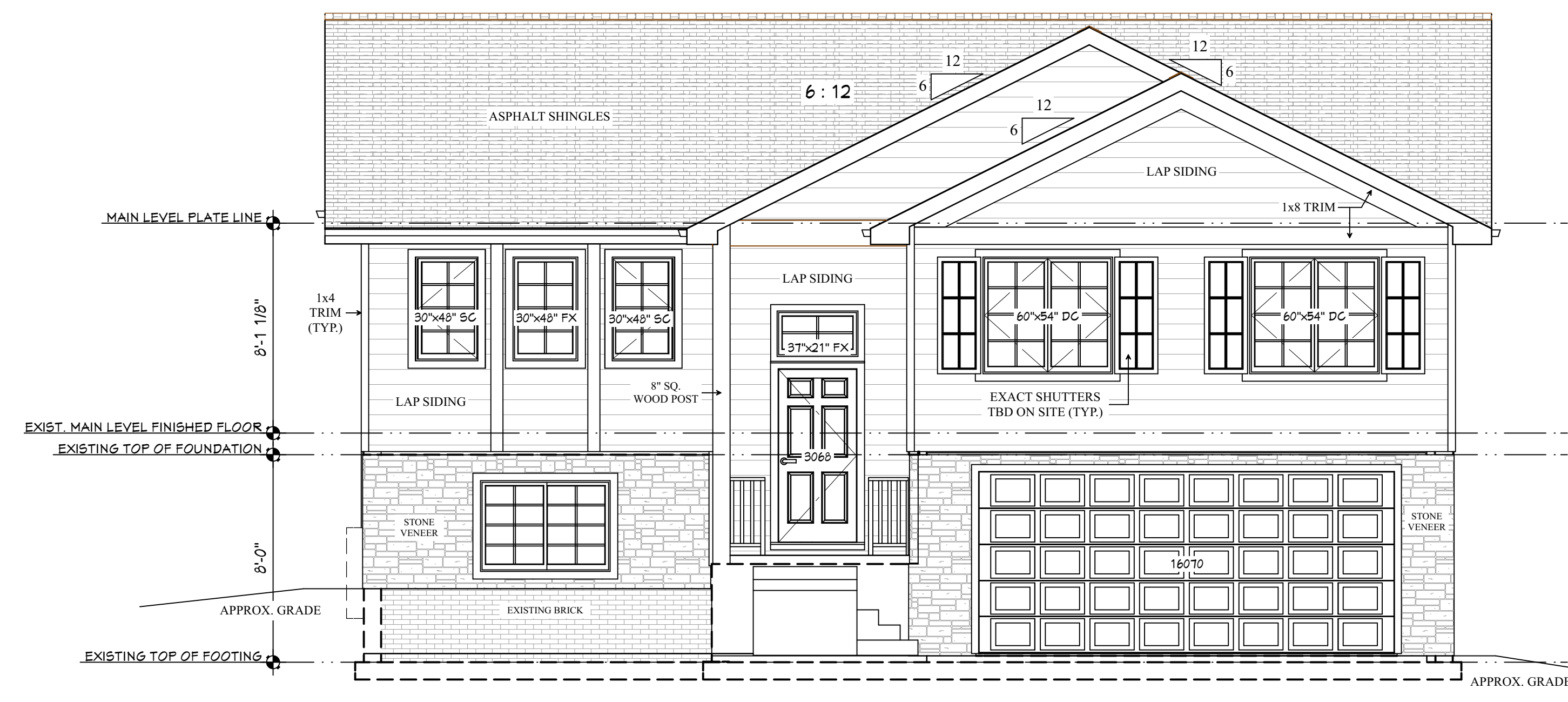
FRONT ELEVATION SCALE: 1/4" = 1'-0"
